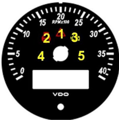
Fig. 4.4: Layout of the tell-tales in gauges with 80 mm and 100 mm diameter.
